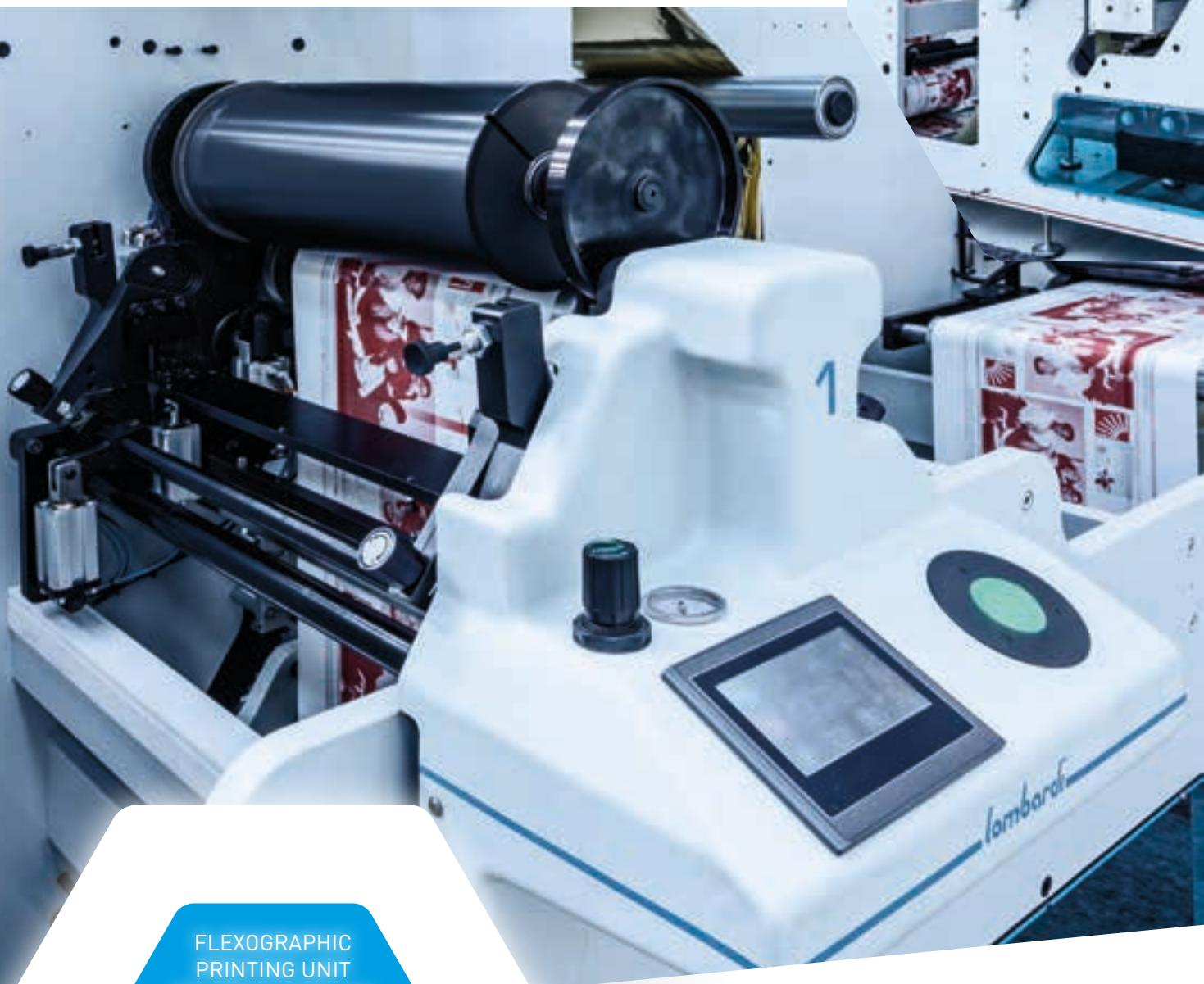
FLEXOGRAPHIC PRINTING UNIT EQUIPPED WITH AN INNOVATIVE PAPER RECOVERY SYSTEM THROUGH A LINEAR CARTRIDGE THAT ALLOWS THE USE OF A SINGLE CYLINDER FOR ALL PRINTING FORMATS.
